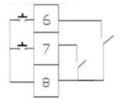
Start connect to the 6&8. Stop connect to 7&8. Separate the 7 & 8 connect again the meter restart again and start from the stop state.
