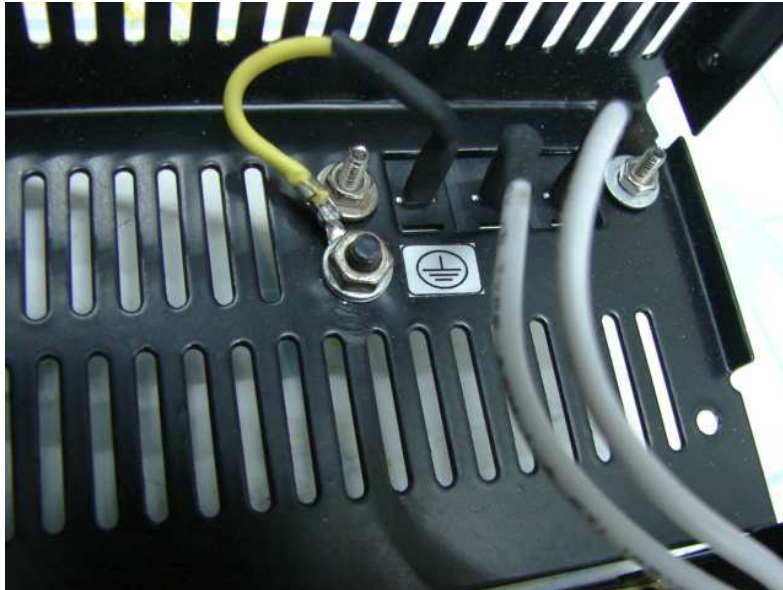
Figure 7 (earth connection -view)
