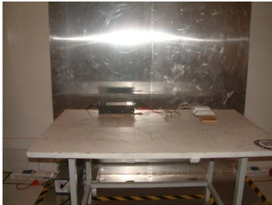
7.1. Photo of power line conducted emission measurement (C.E.)
