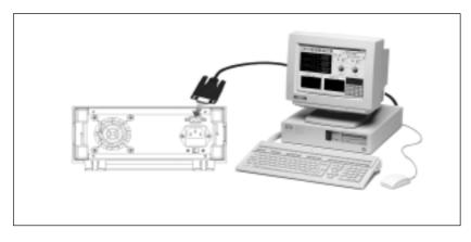
Fig 7 Connect the power supply with PC
