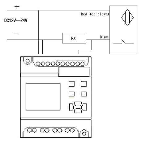
To the same type approach switch, its connection principle is alike. For NO and NC type approach switch, their difference is output relation when it near to
