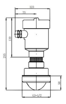
Normal temperature pipe threaded connection
