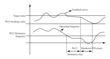
Example: PID action set point is 60% (0 – 100% is corresponding to 0 – 10V), and the wake-up value is 80%, which is actually corresponding to 0 – 10V, then the actual wake-up value is  $60\% \times 80\% = 48\%$  (corresponding to 0 – 10V).
