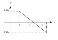
Example 2, upper computer output 4-20mA, and controls running of inverter Output frequency is 100Hz-0Hz
