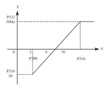
Introduction: P300=2 AV minimum voltage input: 2V (inverter regards signals below 2V as invalid signals):
