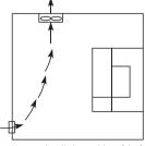
Incorrect installation position of the fan
