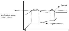
100% current is the rated current of inverter, when P409 is set to be 0, then accelerating torque limit is invalid, and it does not have protecting function.
